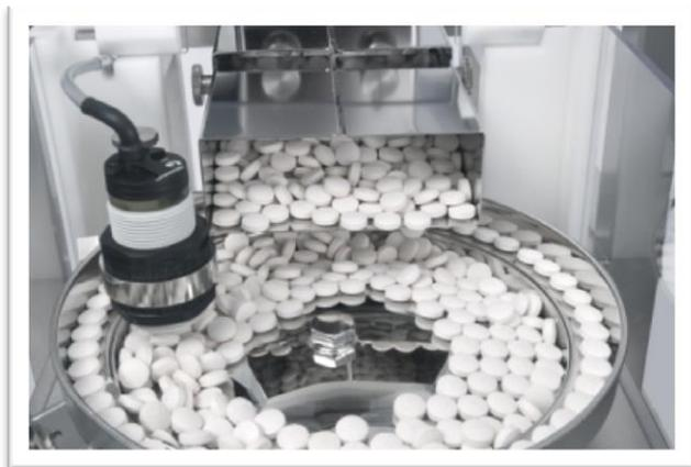
The tablets were around 14mm in length and weighed approximately 1100mg. Some 750,000 tablets were weight sorted at a rate of 15kg per eight-hour shift, with the sorter operating 24 hours per day.
